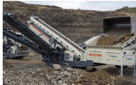
Large feed box allows closed circuit process.
