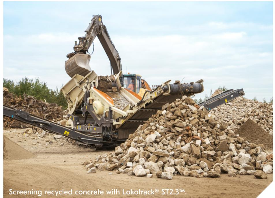
Screening recycled concrete with Lokotrack® ST2.3™.
