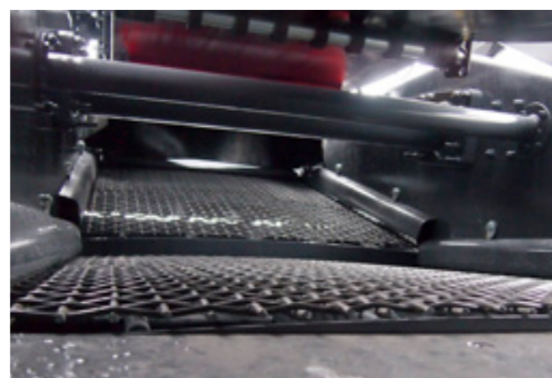
The dual-slope screen enables efficient and accurate separation.
